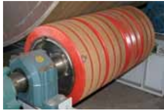
WP-10-900-00200 HUB ASSEMBLY - COMPLETE WITH POWER LOCKING DEVICE; WITHOUT SHAFT
