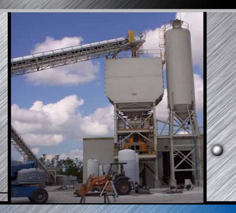
Mixers can be mounted on independent mixer support frames or beneath cement silos.
