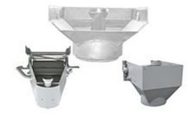
**Truck collection hopper:** 24", 30" & 36" hoppers mounted on the discharge end of the customer's transfer conveyor. The hopper constructed of 1/4" steel, lined with 1/4" 400 brinnell A/R steel. Additional "bolt in" replaceable A/R plates on two sides. Cement enters truck surrounded by rock and sand which is surrounded by water. Note: Any size custom built hopper available consult factory for details. Special liners are also available.
